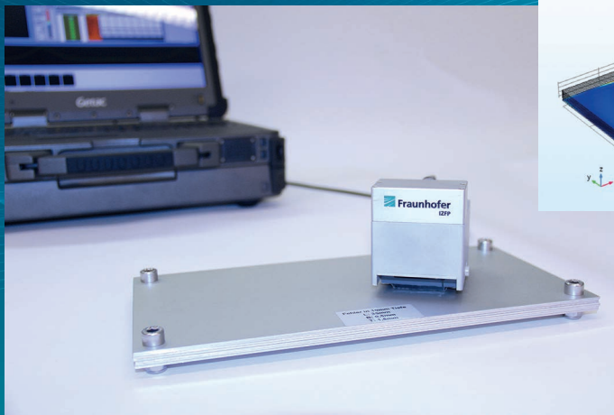
DeepFlawDetector (sensor) and simulation result for sensor development
