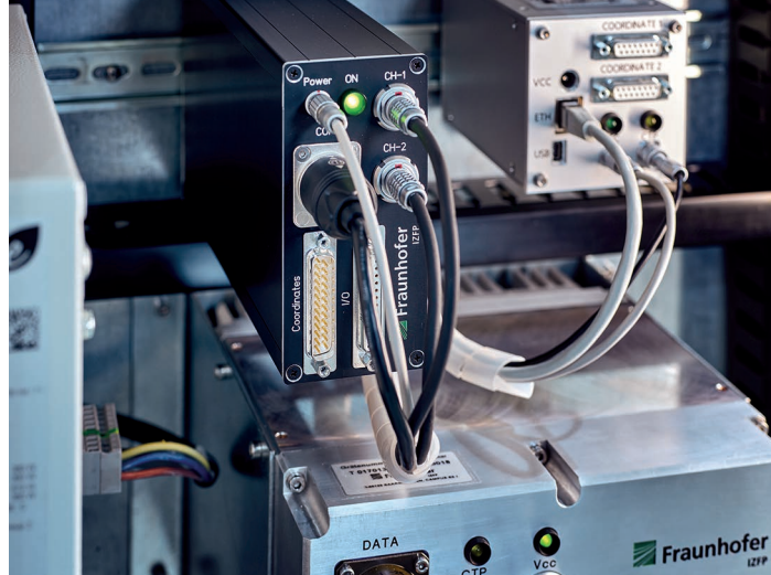
3D SmartInspect leads the way into the digital NDT world: AR system for manual component testing with automated documentation in DICONDE
