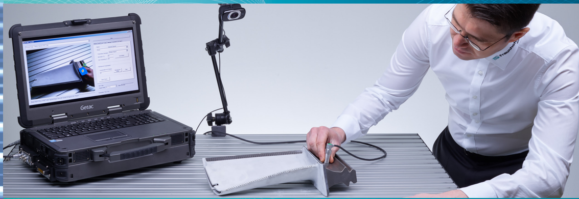
3D SmartInspect – a Fraunhofer IZFP tool for the digital NDT world: Augmented Reality System as a support for the manual inspection of components or large surfaces
