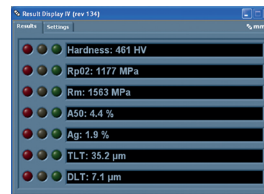
Result of a 3MA inspection
