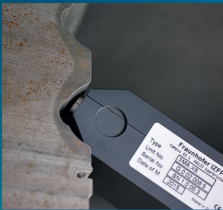
Case depth determination by 3MA-X8
