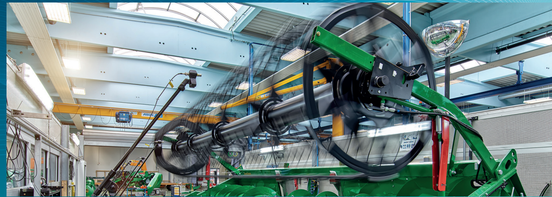
AcoustiX – acoustic sensor system, here on a combine cutter bar
