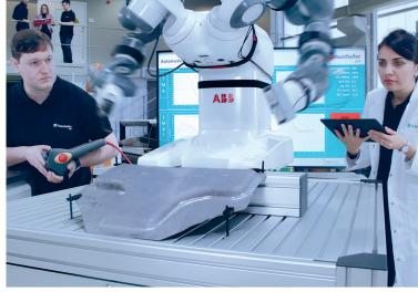
Testing CFRP components using sampling phased array
