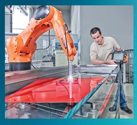
Nondestructive testing and characterization of lightweight construction materials
