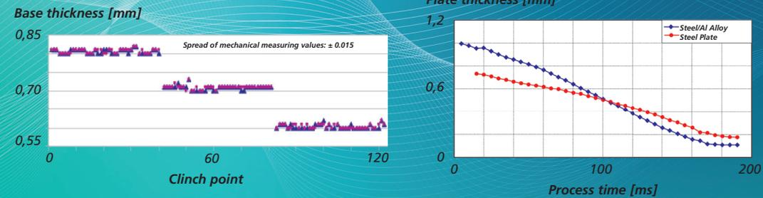
Left: Offline determination of base thickness of joint Al plates; right: Decrease of base thickness of die-sided plate during clinching process
