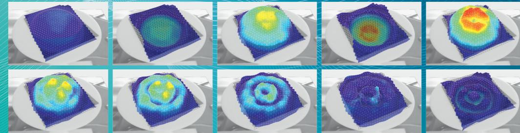
Time measurement: Vibration behavior of a circular air-coupled ultrasound ceramic at different times due to a periodic excitation with 180 kHz
