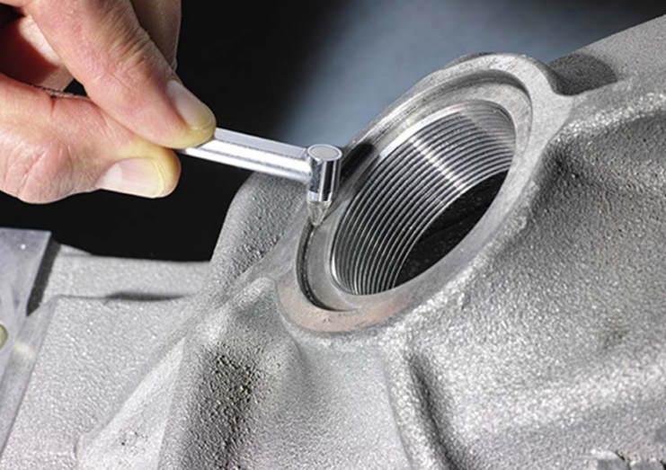
left: Ultrasound sensor for sampling small radii using a contact method; middle: Setup for manipulator-controlled ultrasound testing using a contact method
