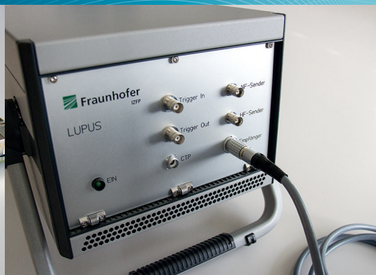
UNIUS board and application LUPUS (air-coupled ultrasound pulser)
